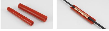
Jiffy Splices are a unique, field-serviceable alternative to permanent splices. Made from the same high quality silicone elastomer as DEUTSCH industrial connector seals and grommets, the Jiffy Splice body houses a contact retention system that secures a mated pair of contacts in a compact environmentally sealed unit.
